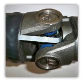
Driveshaft: The WISER system shown here is mounted to the end of the driveshaft, with the strain gauge attached along the shaft itself. Several driveshaft applications require long term testing. With a 1000 mAh Li-Poly battery, the system has been used to obtain over 200 hours of 2kHz data before needing to be recharged. Recharging is accomplished overnight, and the system is sent out again.
