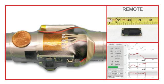
The TECAT WISER Model 4000 torque measurement and monitoring system is a wireless data acquisition system for measuring live torque. It is small, light, power efficient, easy-to-use and non-invasive. The wireless system has the optional ability to measure 3-axis acceleration, pressure and temperature all within the same incredibly small footprint.
