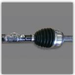
Halfshaft: Measuring torque output to the wheels helps automotive engineers understand torque losses throughout the engine and driveline system. This application requires a durable system, as testing often includes revving the engine and dumping the clutch, sending high load spikes through the halfshafts. In this example, the system is mounted with high strength fiber tape.
